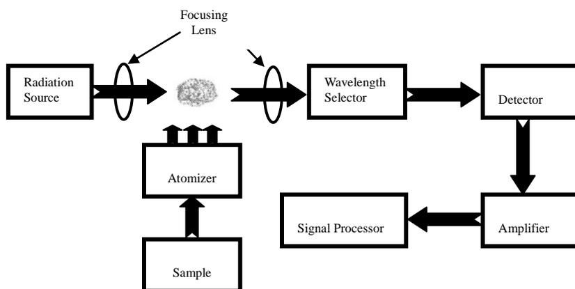
**Figure 6.6** Schematic diagram of atomic absorption spectrometer.
