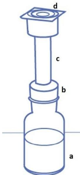
**Figure 6.2** Schematic diagram of the apparatus used in Gutzeit's test. a) A glass bottle containing arsenic, zinc and sulfuric acid; b) rubber with bore; c) narrow glass tube containing glass wool impregnated with lead acetate; d) a filter paper at the top of the glass tube containing either silver nitrate or mercuric chloride.
