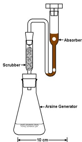
**Figure 6.4** Schematic diagram of arsine generator.
