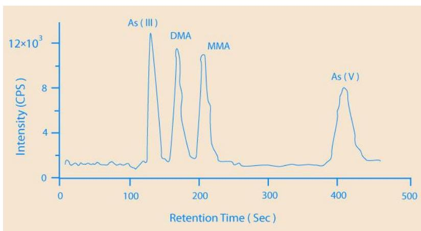
**Figure 6.7** Speciation of arsenic using HPLC-HG-AFS (Le, 2001).
