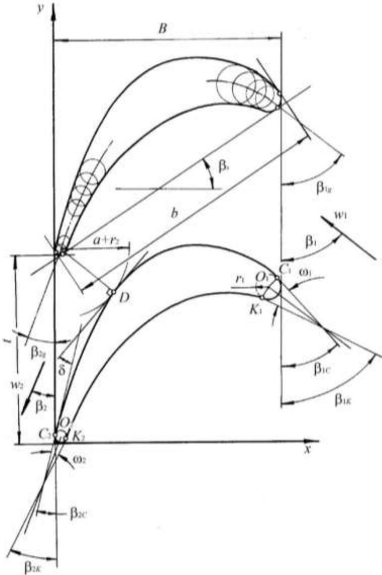
**Figure 5.1** The design parameters of the profile cascade.
