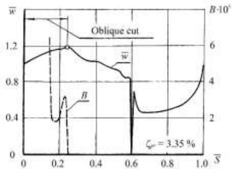
**Figure 5.7** Distribution of velocity and Buri separation criteria  $B$  along the IMPL profile contour. Calculated profile loss coefficient  $\zeta_{pr} = 3.35\%$ .
