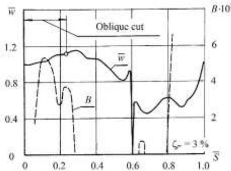
**Figure 5.8** Distribution of velocity and parameter  $B$  along the IMPL profile contour. Calculated profile loss coefficient  $\zeta_{pr} = 3.0\%$ .
