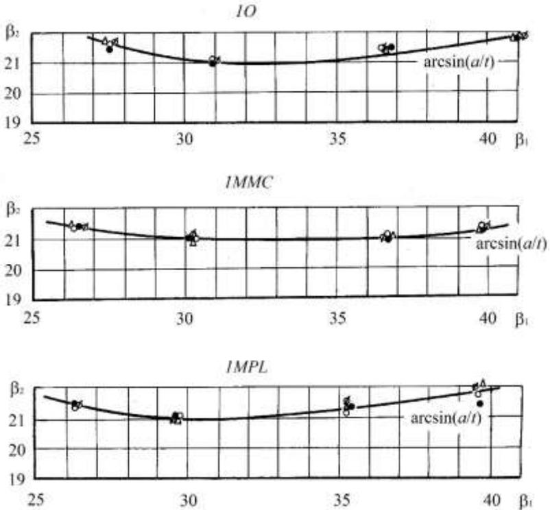
**Figure 5.10** Test results of cascades 10, IMMC and IMPL at different Mach numbers:  $\Delta$  –  $M_{2T} = 0.37$ ;  $\odot$  –  $M_{2T} = 0.45$ ;  $O$  –  $M_{2T} = 0.51$ ;  $\bullet$  –  $M_{2T} = 0.59$ .
