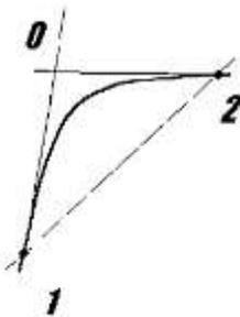
**Figure 5.2** Construction of Bezier curve by 2 points.
