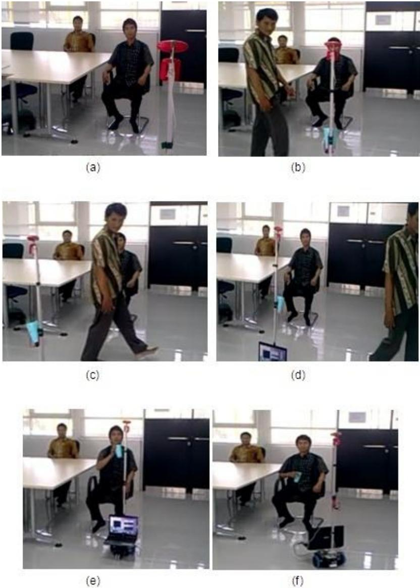
**Figure 11.9** Result of moving obstacle avoidance using stereo vision and Bayesian approach. Sequence action of service robot shown from (a) until (f) to deliver a cup to an identified customer and go back to home.
